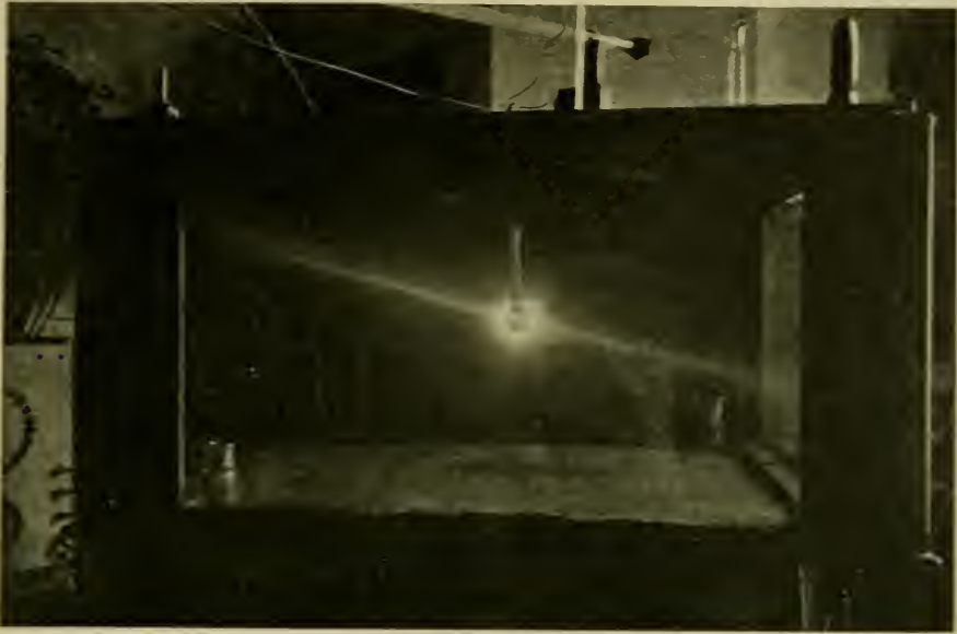
Fig 2. Lamina of corpuscle rays in the plane of the magnetic equator of a magnetic sphere serving as cathode.
